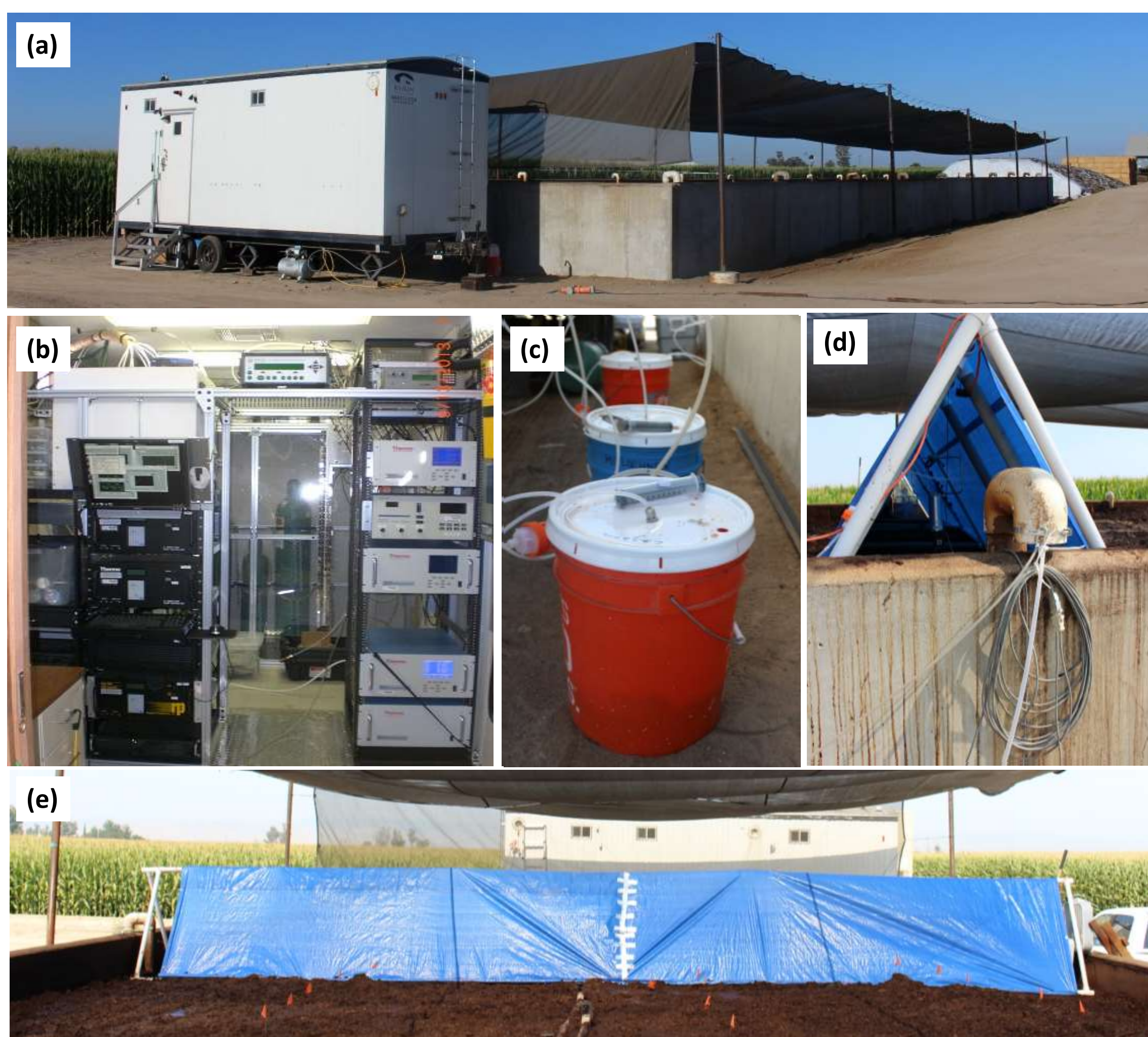
Figure 5. Sampling methods. (a) Mobile Agricultural Air Quality Lab parked next to the vermifilter, (b) Gas analyzers in the MAAQ Lab, (c) flux chambers for gas measurements from L, I, and E, (d) setup for B gas measurements, (e) triangle sampling tunnel for S gas measurements
