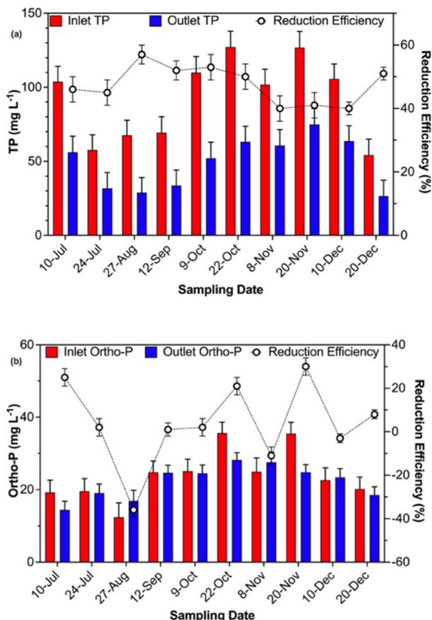
Fig. 5. Bar graphs present influent and effluent concentrations of total phosphorus and orthophosphates, while the line graph shows the corresponding reduction efficiencies, during the study-period.
