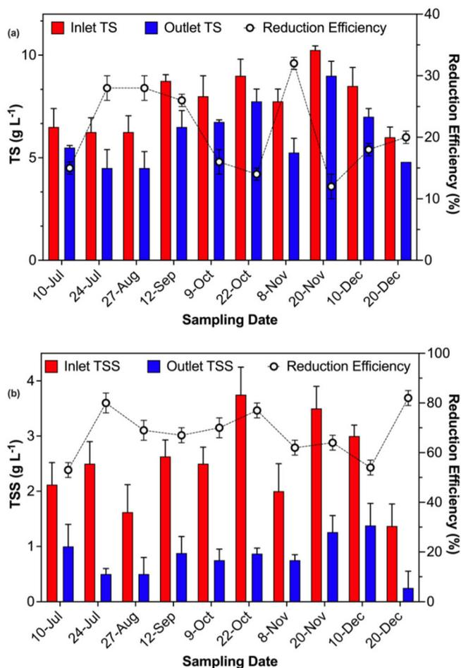
**Fig. 2.** Bar graphs present influents and effluents solids concentrations: (a) total solids (TS) and (b) total suspended solids (TSS), while line graph presents the corresponding reduction efficiencies, during each sampling event.
