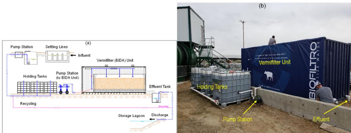
**Fig. 1.** A schematic (a) and a photo (b) of the vermifiltration system used in this study.
