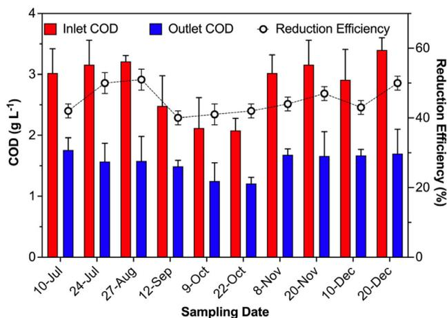
**Fig. 3.** Bar graphs present influents and effluents chemical oxygen demand concentrations, while line graph shows the corresponding reduction efficiencies, during each sampling event.
