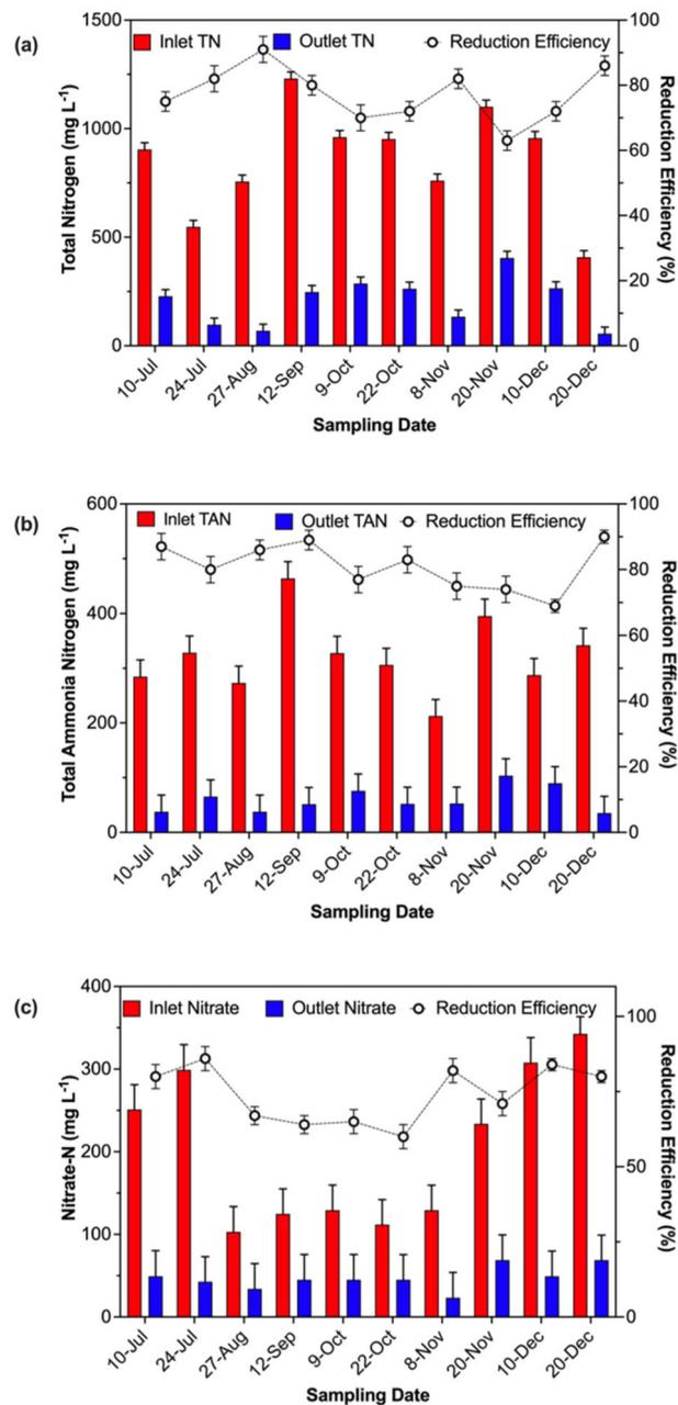
**Fig. 4.** Bar graphs present the concentrations of total nitrogen (TN), total ammonia-nitrogen (TAN), and nitrate-nitrogen (nitrate-N) in the influents and effluents, while line graph presents the corresponding reduction efficiencies during the study period.
